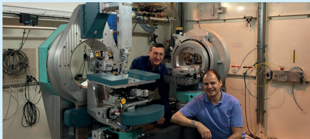
The newly installed diffractometer at beamline ID10, which will allow faster data collection.
