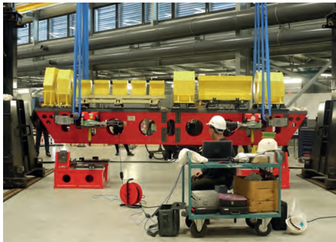
Mechanical technician Marc Lesourd measures the acceleration as the prototype girder is lifted to test for movement of the attached dummy magnets.
