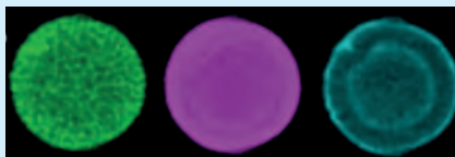
Reconstructed images of cobalt phases in mm-sized samples observed under reduction of a cobalt catalyst precursor.
