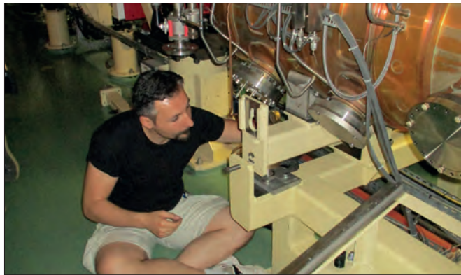
RF engineer Alessandro D'Elia with one of the additional cavities installed in the booster to improve the efficiency and reliability of the injector complex.
