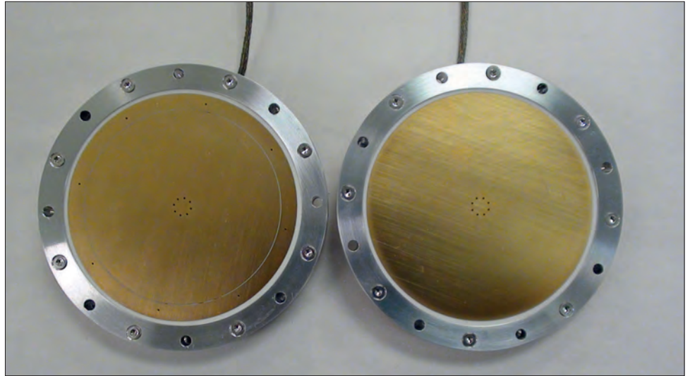
NCG-1-AL-UHV capacitive sensors.
