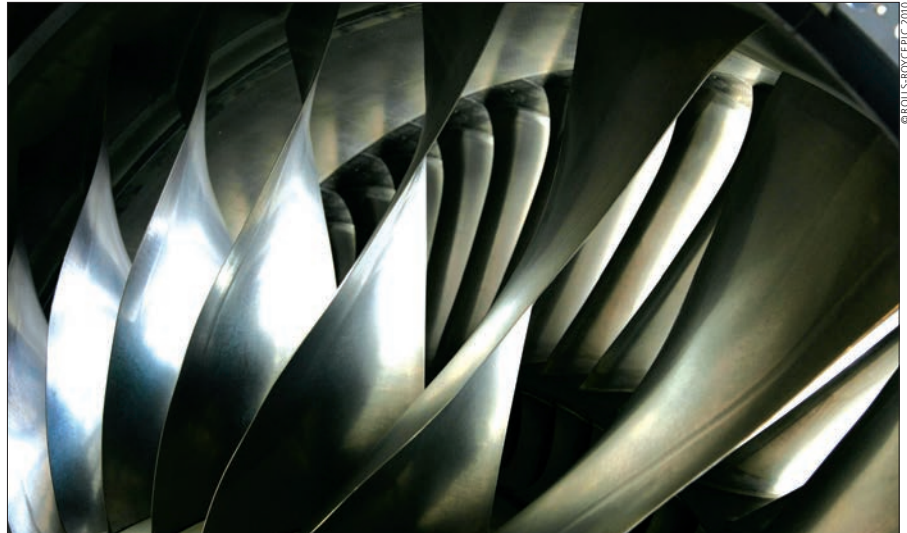
The unique titanium wide chord fan blades, seen here on a Trent 900.
