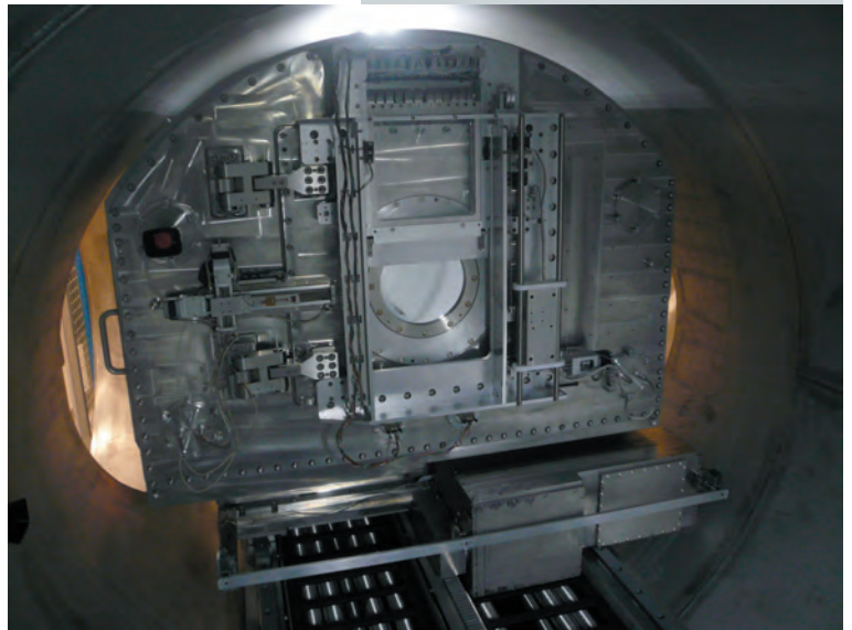
Fig. 3: ID02 detector wagon (front view) inside the USAXS tube.
