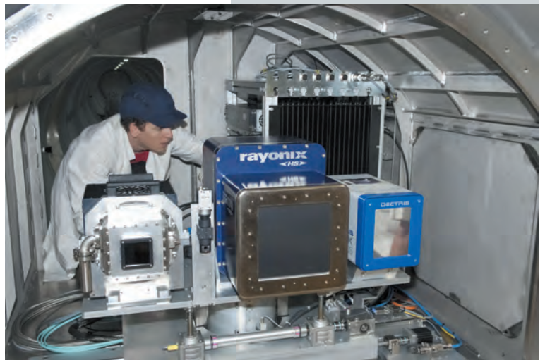
Fig. 4: Detectors inside the ID02 SAXS conveyor: FReLoN camera, beam viewer, Rayonix MX170 CCD detector, Pilatus 300K hybrid pixel array detector (from left to right).
