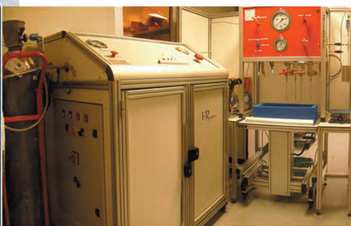
Fig. 148: a) Phase diagram of water. Unprotected crystals cooled at ambient pressure (AP-cooled) produce crystalline ice. At high pressure the solvent is transformed into HDA-ice. b) High pressure cooling installation at beamline ID23.
