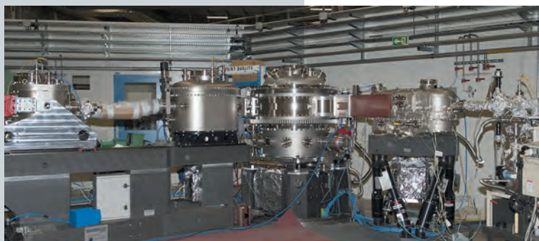
Fig. 2: ID32 RIXS branch: refocusing optics, sample chamber, collimating optics and grating vessel (from right to left).
